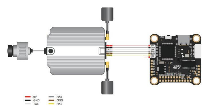
Work with Vista VTX by soldering
