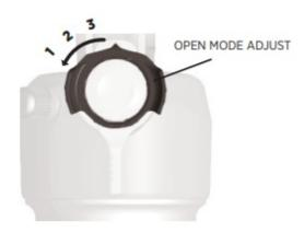
Open mode adjust provides 3 additional fine tuning adjustments for the OPEN mode.
