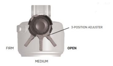
The **3-position** lever is useful to make on-the- under significant changes in terrain, and is intended to be adjusted throughout the ride.
