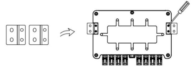
Choose the place you want to install the S-Box Plus. Place the S-Box Plus on the wall and mark the position of the 4 holes from fixing blocks.
