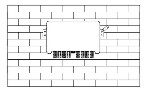
Drill holes with electric drill, make sure the holes are at least 50mm deep, and then tighten the expansion tubes.
