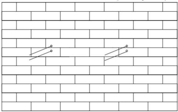
Insert expansion tubes into the holes and tighten them. Install the fixing blocks with expansion screws.
