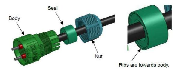
**Step 3:** Tighten wires as shown in the figure below. Tightening torque 0.6±0.1N·m, then insert cable respectively to pin hole.
