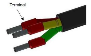
Step 2: Insert the parts into the cable.
