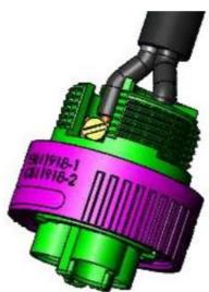
Step 4: Screw body to housing, tightening torque 1.2±0.2N·m.
