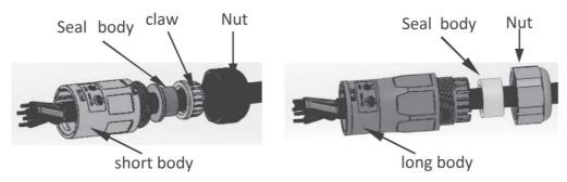
• Crimp wires, screw twisting torque 0.8+/-0.1N-m.
