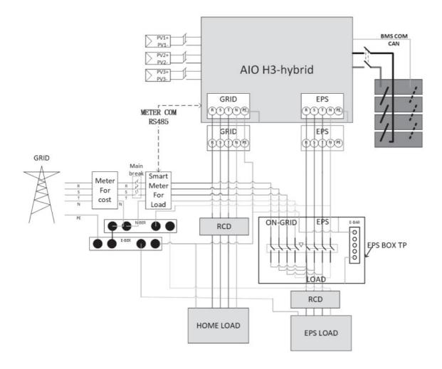
This diagram is an example for an application in which neutral is separated from the PE in the distribution box.
