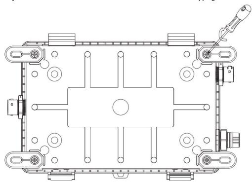
**Step 2:** Use EPS Box -TP with cushion blocks as a template to mark the four holes' position on the wall with marker pen.
