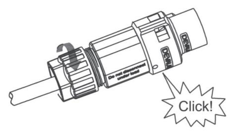
• Remove the ON-GRID connector: Press the bayonet out of the slot with a small screwdriver or the unlock tool and pull it out, or unscrew the threaded sleeve, then pull it out.
