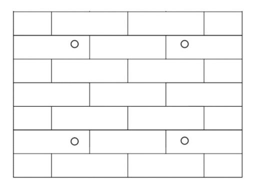
**Step 3:** Drill holes with (') 6 driller carefully, make sure the holes are deep enough for installing. Install the expansion tubes through cushion blocks into the holes and tighten them.
