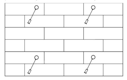
Step 4: Install the expansion screws with screwdriver to fix the EPS Box-TP.
