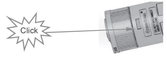
Put the sealing body and yarn trapper into the main body, screw the lock nut into the main body, and the torque is (2.5 + / - 0.5N-m).
