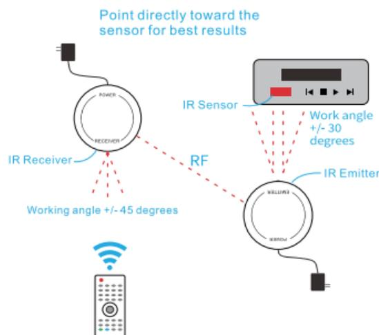
**Step One:** Plug the power adapter and connect it to the Infrared Receiver and the Infrared emitter via the USB power cables, the LED indicator of the receiver and the emitter will blink twice.
