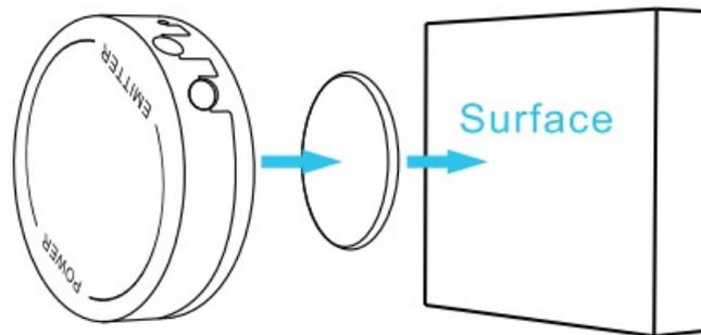
To keep the IR Infrared receiver and emitter in one place, we have included adhesive.
