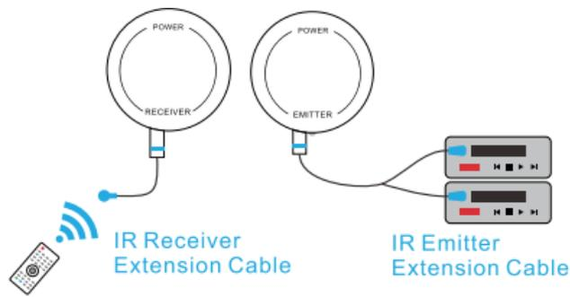
**Step One:** If you want to extend the reach or hide the IR receiver, connect the IR Receiver Extension Cable to the device.
