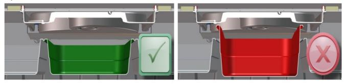
Do NOT block the fan airflow
