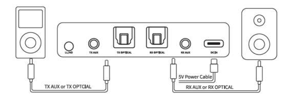
Use the BYPASS function if your TV only has ONE OPTICAL Output which is currently occupied by your AV receiver or soundbar. Toggle between BYPASS and Bluetooth mode using a simple switch. No need to unplug any cable. In Bypass mode, BTO5 can be used as a decoder to convert audio between 3.5mm AUX and optical output.
