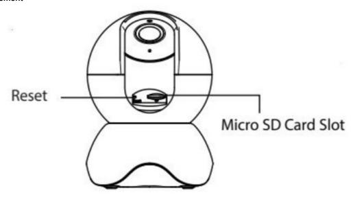
The record files of the IP camera can be stored in the Micro SD Card.
