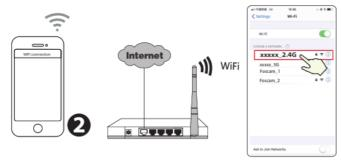
**Tips:** You need to connect to the 2.4GHz network if your WiFi router is dual-band—most newer routers have both 2.4GHz and 5GHz channels. For example, choose SSID: XXXXX\_2.4G.
