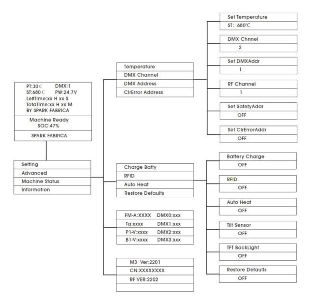
**NOTICE** Press <OK> to enter the menu setting. The screen will automatically return to the main state interface with no modification.
