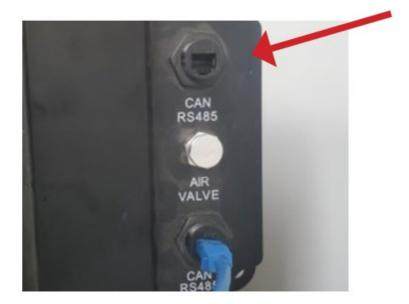
4. Connect the jack end of your Communication Cable to the empty "CAN RS485" port of your eFlex battery.
