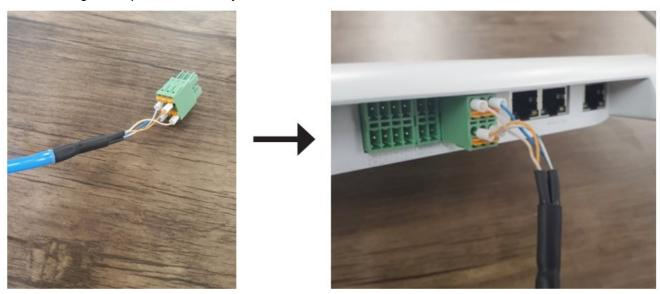
3. One of your eFlex batteries will have a plug in the port marked "CAN RS485".
