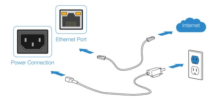
Connect your device to a power outlet and an Internet connection. This is usually a modem, but could also be another device on your network.
