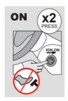
Do not press the brake pedal. Press twice the to turn on the ignition.
