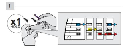
Press hold and the programming button: Connect the 4-PIN Data-link harness (Black connector).
