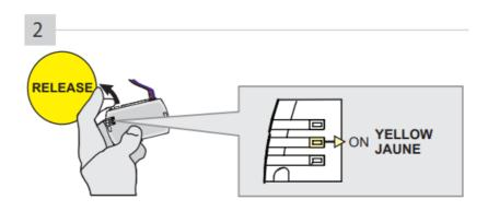
If the LED is not solid YELLOW the 4-Pin connector Release the programming button when the LED is YELLOW disconnect.
