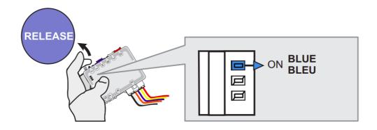
If the BLUE LED is not ON soli disconnect the 6-Pin Main connector and go back to step 1.
