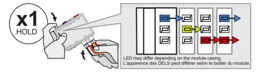
Release the programming button when the BLUE LED i ON.
