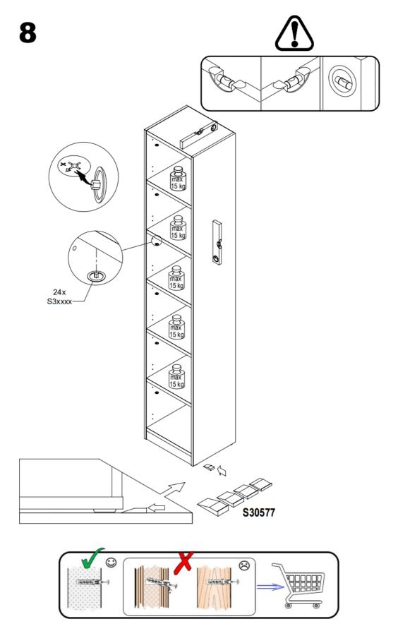
Before suspending or fixing furniture to the wall (in order to prevent falling over), check the type and strength of the wall. Select wall plugs and screws appropriate for the given type of the wall. In the case of doubts, contact a specialist. The installation must be performed by a competent person.
