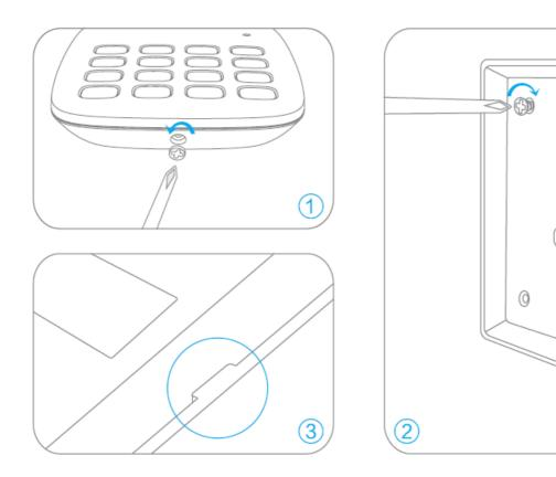
**Note:** Because of the tamper switch, opening the rear cover of the keypad, when the system is armed will trigger the alarm. In such an instance, to stop the alarm, disarm the system.
