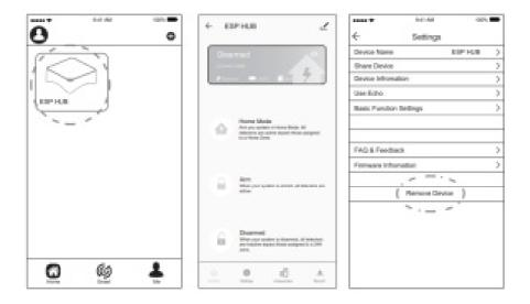
Turn the Control panel on, press the "Connection Button" 5 times, within 5 seconds of the Hub being turned on, the Hub will then be restored to factory settings. The system settings and all connected accessories will be restored.
