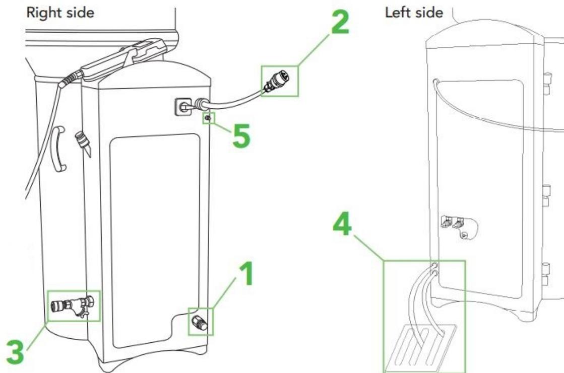
6. Mount and connect raceway, antenna and suction point
