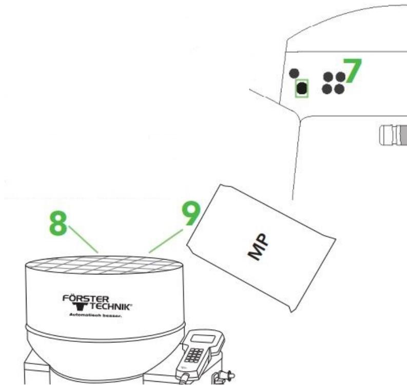
11. Switch on vapour screen for powder outlet if available
