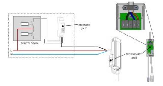
The mains power cable for Shuttle® is no longer required.
