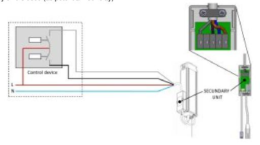
When an power outlet or other constant Live and Neutral are available near the Shuttle®, the motor can also be powered directly from the outlet. The power plug, attached to the secondary unit, can then be removed.
