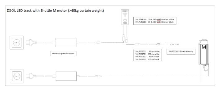
The 24V power adapter used for DS XL LED systems is always the Shuttle M adapter set:
