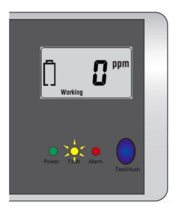
The normal standby time of battery is 3 years minimum. If there is problem with the battery or low battery signal warning keeps for over 30days, please replace the battery timely. It is recommended to use the same type of battery when changing the battery 3 xLR6 SIZE AA 1.5V battery).
