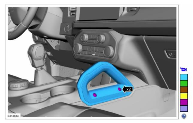
6. Remove the screws, release the clips and position the lower center instrument panel trim panel.
