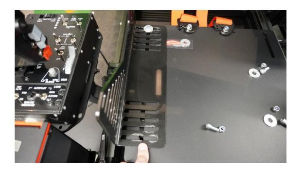
Now measure the required seat inside width and align the seat brackets. Then screw on the other side (front or rear). Again, adjust the seat slider as required. Do not tighten these screws either.
