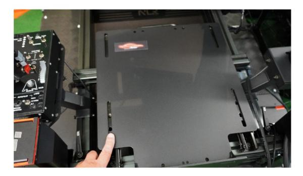
Now prepare the required screws. First fasten the front straps (not included). To do this, use 2x M8x20 cylinder head screws with 4x M8 washers at the top and bottom and 2x M8 lock nuts. Align the belt buckles and screw tight. The eyelets are optional and can be used to hook in the rear seat belts (see original BT1 manual).
