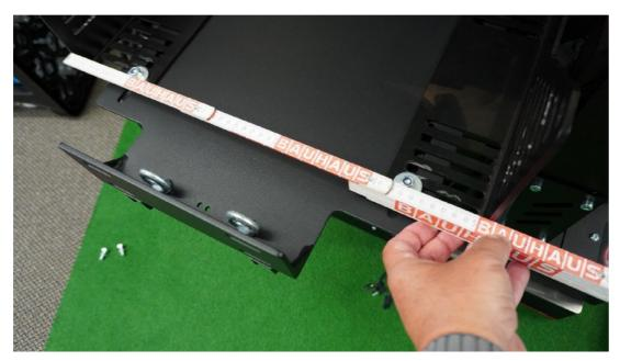
The seat can now be inserted, the desired angle set and the screws inserted (not included in the F2MBT1 set but in the other product sets). Attach the two corner straps directly. If necessary, use longer M8x30mm screws.
