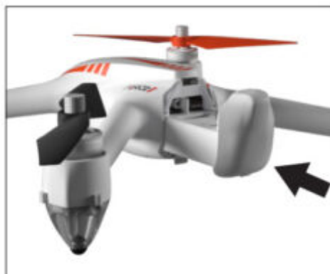
SLIDE BATTERY IN COMPARTMENT
