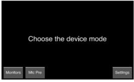
**Mic Pre** – Accesses the hardware controls of a remote device.
