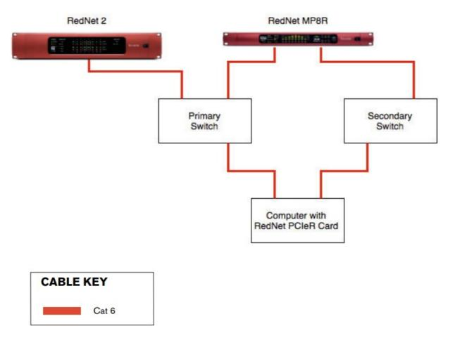
RedNet units with only one network port must be connected to the Primary Switch Only. RedNet units must be set to Redundant Mode in Dante Controller in order for this setup to work, otherwise Switched mode will only daisy chain devices.
