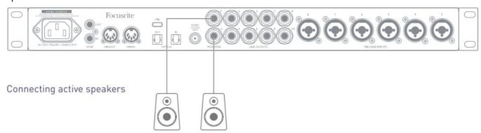
All the line output connectors are 3-pole (TRS) 1/4" jack sockets, and are electronically balanced. Typical consumer (hi-fi) amplifiers and small powered monitors will have unbalanced inputs, either on phono (RCA) sockets, or via a 3.5 mm 3-pole jack plug intended for direct connection to a computer. In either case, use a suitable connecting cable with jack plugs at one end.
