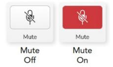
When Mute is on, the hardware buttons: Auto Gain and Mute light red, and the Gain halo on your Vocaster pulses red.
