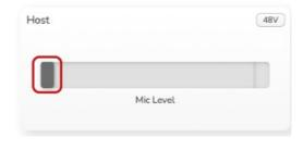
You can click and drag the slider in the software to increase the gain (right) or reduce the gain (left). When you move the hob the slider will move to reflect this.
