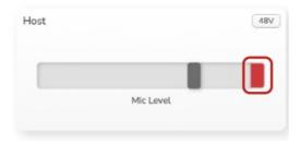
If you see the clip meter appear, turn down the whole whose the Slider to the left to reduce the gain. To 'clear' the Clip Indicator, click the red Clip Indicator itself. This removes the light for all inputs and Mix channels.
