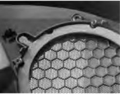
Fix the Focal speaker (use the original screws).
