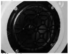
Focal speaker riveting (aluminum 4x16mm rivet).
