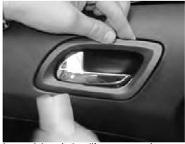
Use the same tool to dismantle the bar and the window lifter command.
