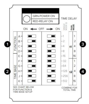
**Example:** In the example shown, delay time has beenset to 5 minutes and run time is set to 20 minutes.
