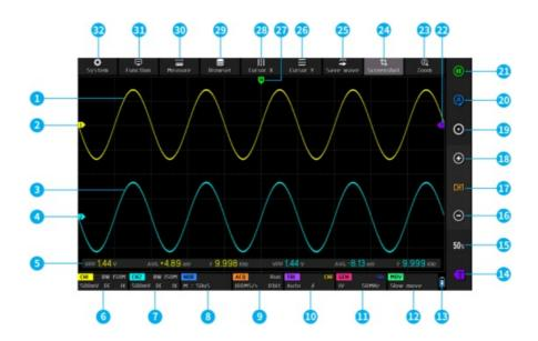
①The signal waveform of channel 1 is displayed in yellow brightness when the color temperature is turned off. The brighter the area, the greater the probability of the area
