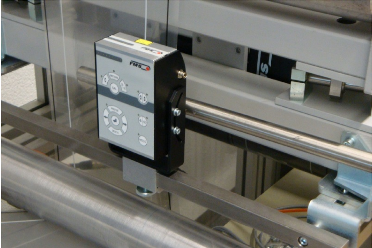
Fig. 2: Mounting of sensor on the square bar, view of tilting device
