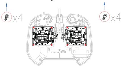
4. Switch the gimbals to the oppsite side and make sure the gimbals have been rotated 180 degrees, then tighten the srcews removed before.
