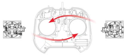
5. Reattach the front cover and back cover, and tighten the screws.
