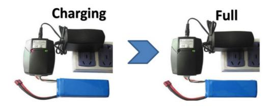
When the charger is not charged, the green light will be on; when it is charged, the red light will be on; when it is full, the red light will be off
