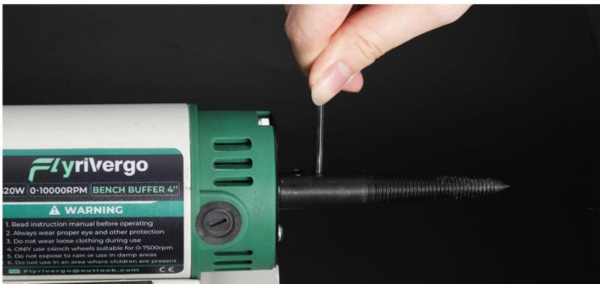
3. Put the cotton wheel on the spindles. After making sure the wheels are stable, you can start your polishing work.
