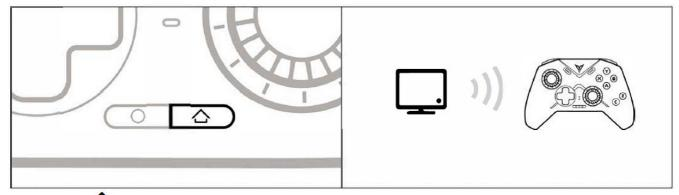
Press the  $\triangle$  button on the controller, and it will automatically connect. The indicator light will stay white.
