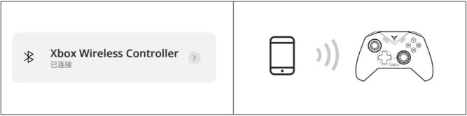
Turn on the device's Bluetooth.con- necto the Xbox Wireless Controller, and the controlle indicator ight keep in whitelight's solid white
