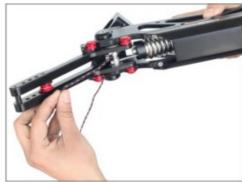
• Now you can hold the Placid arm in its standard position. The cord is aptly set to perform its function. By using an Allen key, tighten the mounting bracket of the Placid Arm with the Flowline support arm.
