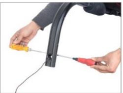
• Turn the Placid Arm upside down. By using an Allen key, loosen the mounting bracket of Arm. Now the bracket has enough space for the cord to pass through it.
