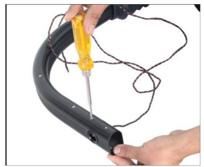
• Pull out the front pulley carefully, so it doesn't drop into the Flowline support bar and Insert the cord from the bottom hole and tug it out from the top hole.
