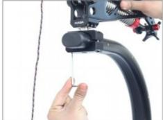
• To fix the Placid arm at its appropriate position, attach one side of the Safety Elastic Cord to a knob on the Placid arm. Then, drag the other side of the elastic cord across the Flowline support arm, and attach it to the knob on another side of the Placid arm.
