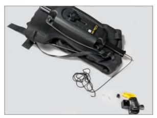
• To detach the extension from the Support Rod of the Vest, remove its screw using a screwdriver.
