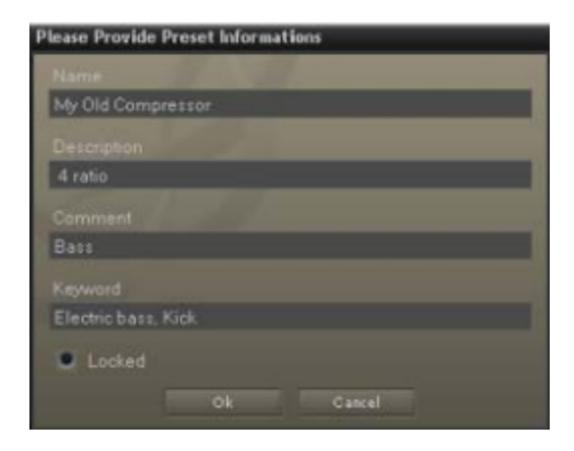
When engaged, the preset is protected, and any subsequent modifications or edits are allowed for the original author only. This comes in handy in a multi-user configuration. Protected presets can of course still be loaded or deleted when the user logs under a different computer session.
