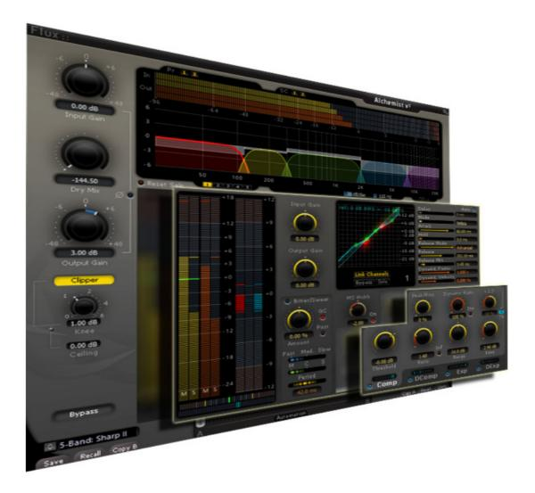
At first, the wideband signal is split into frequency bands by a slope adjustable cross-over.
