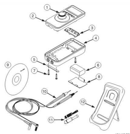
Description Qty. Item Part No. Rotary knob 1. 1618022 1 Case top 2. 1618355 1 Keypad 3. 1 1612222 Case bottom 1 4. 1618005 Non-skid foot 1 5. 885884 Battery. 9 V, Alkaline, ANSI / NEDA 1 6. 614487 1604A or IEC 6LR61 7. Case screws 665098 4 Battery door 8. 665106 1 CD ROM 1 9. 2088974 Test lead set 10. TL75 1 Alligator clips 11. AC72 1 Holster, yellow 12. C10 1
