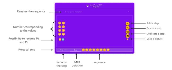
**Step 2** To create a sequence, first one can upload any picture from a directory as a guide to building the protocol. This picture is a reminder to know which part of the chip/microfluidic set-up is connected to which valve.
