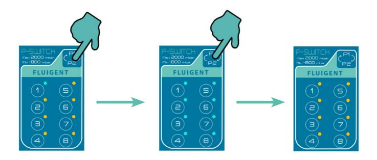
By pressing the "P1 <-> P2" button, one can set every valve at the same time to the same position. By pressing it again, one can set every valve on the second position. (LEDs color indicates the supplied pressure)
