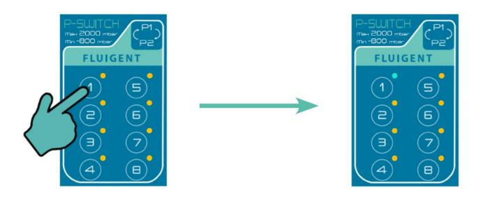
To switch any valve position from P1 to P2 or P2 to P1, press the corresponding button of the valve. Once done, the led will change color either in orange or in blue to indicate the new current position. **Note:** Several valves can be actuated at the same time.
