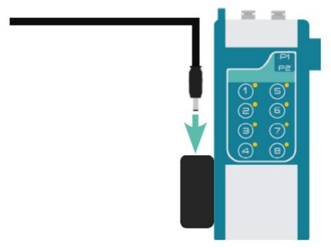
Power ON the module using the LineUp Supply Kit and/or LINK module. Once done, the P-SWITCH LEDs will turn orange, and the default dispense pressure is set on P1.
