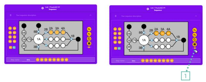
Step 4 Use the right click or double click to change the valve position and edit the step sequence. When the
