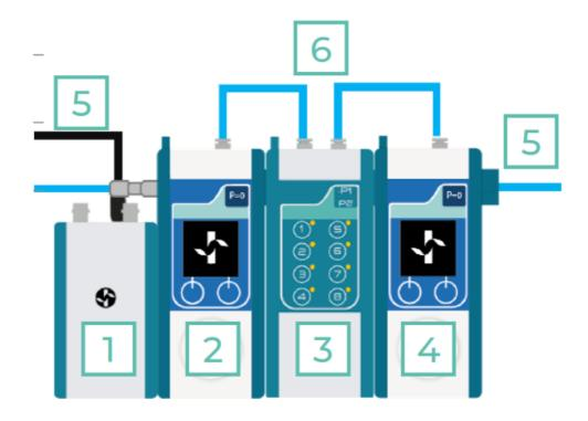
In the configuration above, the LineUp P-SWITCH TM allows one to switch between the P1 regulated pressure or the P2 vacuum both supplied by each Flow EZ TM or Push-Pull.
