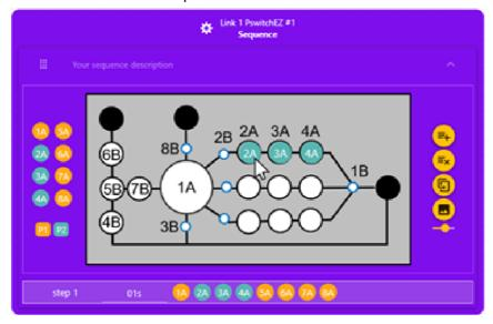
Step 5 To add a step, click on the "add step" button (1) or "duplicate step" button (2) on the right.
