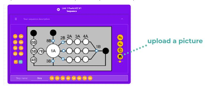
**Step 3** Drag and drop the valve numbers on the picture. By using the slider (1) on the right one can resize the numbers.
