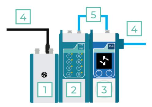
In the configuration above, the LineUp P-SWITCH TM allows one to switch between the P2 vacuum supplied by the negative Flow EZ TM or Push-Pull and the P1 atmospheric pressure.
