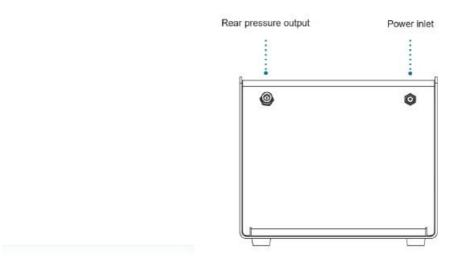
The rear pressure output delivers the same pressure as the front output. One or the other can be used for better tubing management, or both at the same time to pressurize two pressure controllers.
