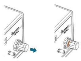
3. Turn the knob to change the output pressure (from 0.1 bar to 2.30 bar) in order to meet the supply requirement of the pressure controller channel range.
