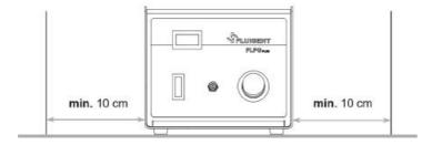
Please, always place the FLPG Plus on a horizontal and stable surface. Keep clear for at least 10 cm at sides of FLPG Plus. This allows for ventilation and the air drying system to function properly.
