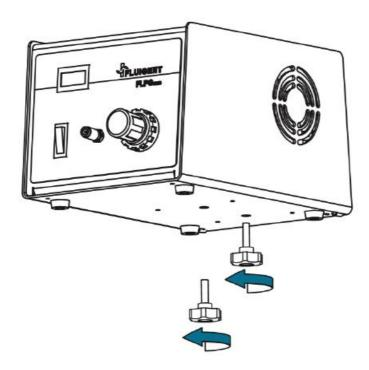
These screws are used to protect the compressor inside during the transport. Please keep these screws in case of future transport.
