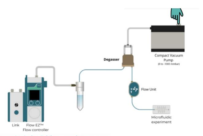
Example of microfluidic setup using Degasser
