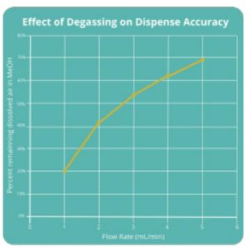
Plot of typical degassing efficiencies using air saturated methanol measured by UV absorbance.
