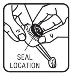
If Replacing Seal: Use only a genuine Fluidmaster 242 seal.
