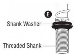
Place Shank washer onto threaded shank of fill valve. Flat side up.
