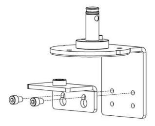
If required change the clamp plate setting by removing the screws and adjusting to correct setting
