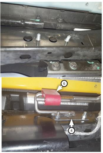
9. Place clamp (5) onto high exit pipe (3) then connect it to mid pipe. Insert wire hanger into rubber hanger then tighten clamp just enough to allow for later adjustment.
