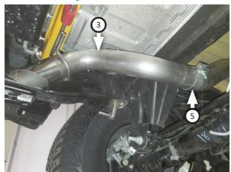
10. Adjust exhaust components for maintaining "clearance and compensating ng for suspension, travel, and vibration then tighten all clamps. Finally, fit (x3) hanger keeper (11,12) onto each sideways hanger.
