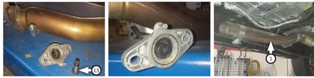
7. Place clamp (5) onto the mid-pipe (2) then route it over the axle and connect it to the inlet pipe. Insert wire hanger into isolater then tighten clamp enough to hold parts.
