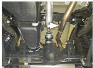
5. Apply to seize compound to threaded fasteners for a more secure install.
