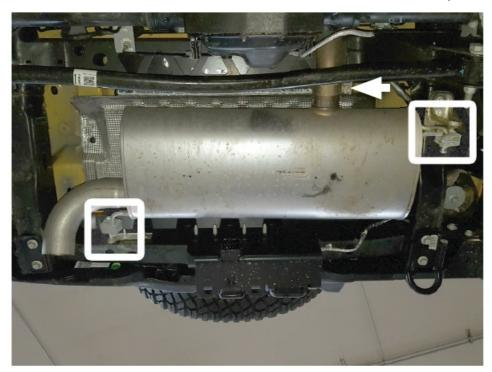
2. Support front pipe then remove fl ange fasteners. Unbolt isolator mount from frame, separate rear wire hanger from isolator then remove front pipe from vehicle.
