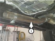
5. Place **clamp (6)** onto mid **pipe (2)** then route itove axle and connect it to inlet pipe. Tighten clamp just enough to allow for adjustment.
