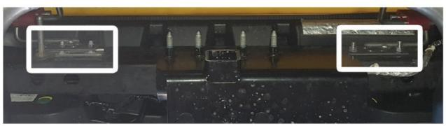
7. Place **clamp (6)** onto **muffl er (3)** then connect it to mid pipe. Insert wire hangers into rubber hangers and ghten clamp enough to allow for adjustment.
